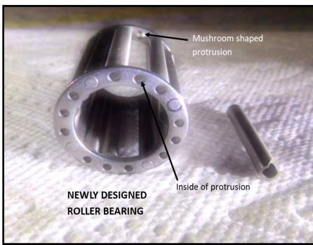
NOTE: the protrusion stamped into the end plate at the rear. Note that what appears to be holes in the end plate at the front are not holes, but are the inside of the protrusion. Note the element on the right, there is a recess drilled into each end. The element end was broken during removal.
